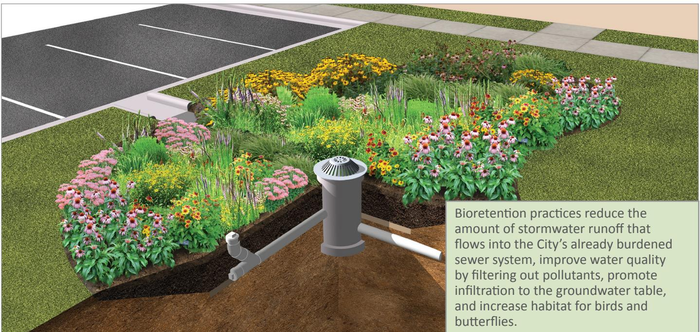
Bioretention practices reduce the amount of stormwater runoff that flows into the City's already burdened sewer system, improve water quality by filtering out pollutants, promote infiltration to the groundwater table, and increase habitat for birds and butterflies.
